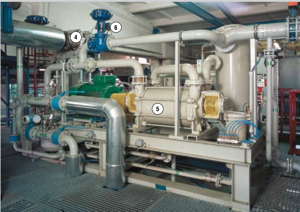
Fig. 11.2: Vacuum pump module for RV23VAC with condenser (4) vacuum pump (5) pressure controller (6)
