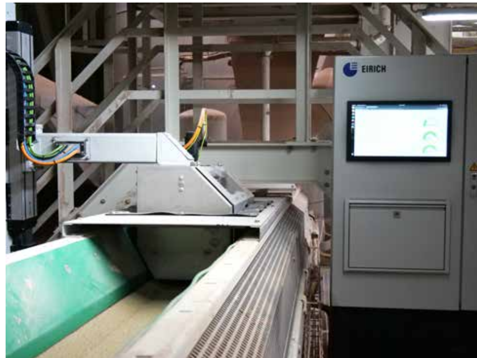
Optical granulate measurement through VC1
